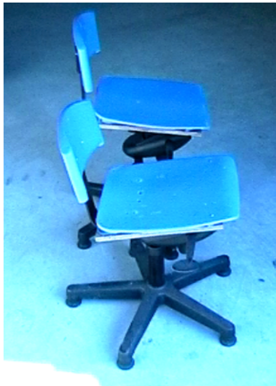
Figure 3.1. Experimental chairs showing range of seat angle adjustment.
